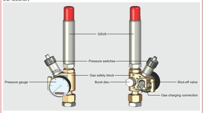
The gas safety block GSB450 consists of a brass block (other materials on request) with an integrated vent valve and shut-off valve and connections for:
